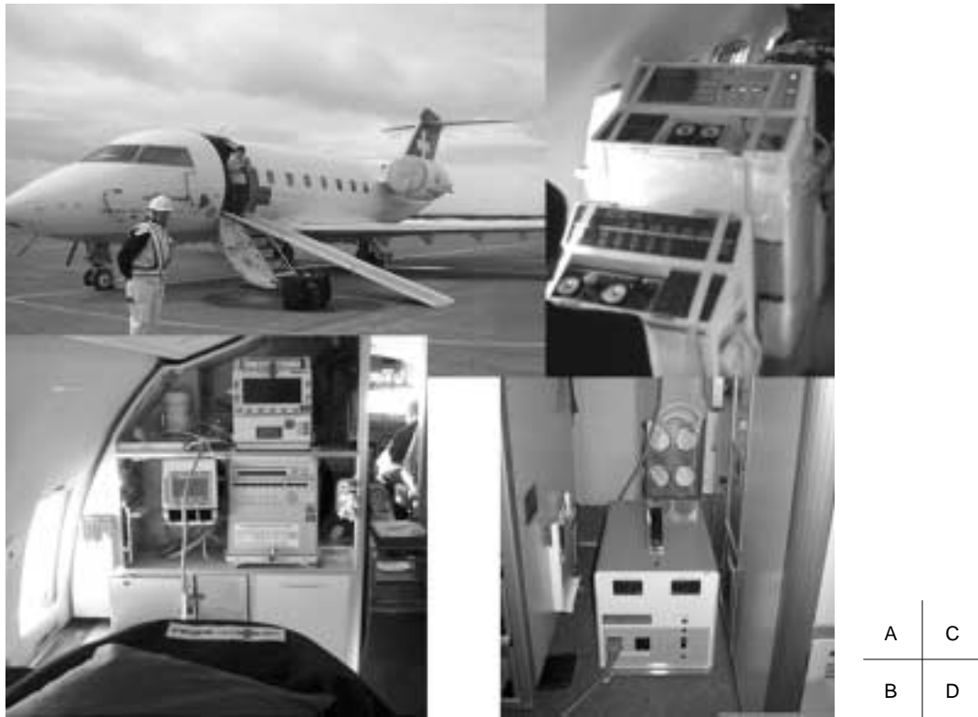
Fig. 2 A Outside of the Rega Air Ambulance. B Inside of the Rega Air Ambulance. C LVAD driving units on the side of the bed in the Air Ambulance. D Down transformer in the Air Ambulance.
